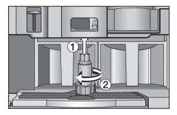
Insert the tool (supplied) up into the unit, ①. Turn it to the left, ②, to loosen and remove the perforator
